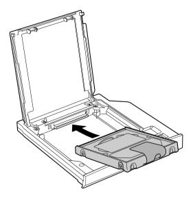
Figure 8-22 Inserting the HDD
